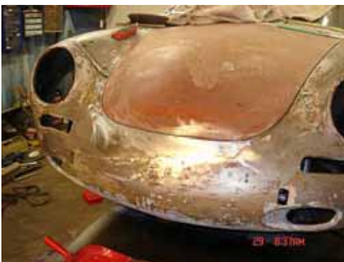
In bare metal condition, this shows Doug Dutton's careful reconstruction of the front end, ca. 2006
