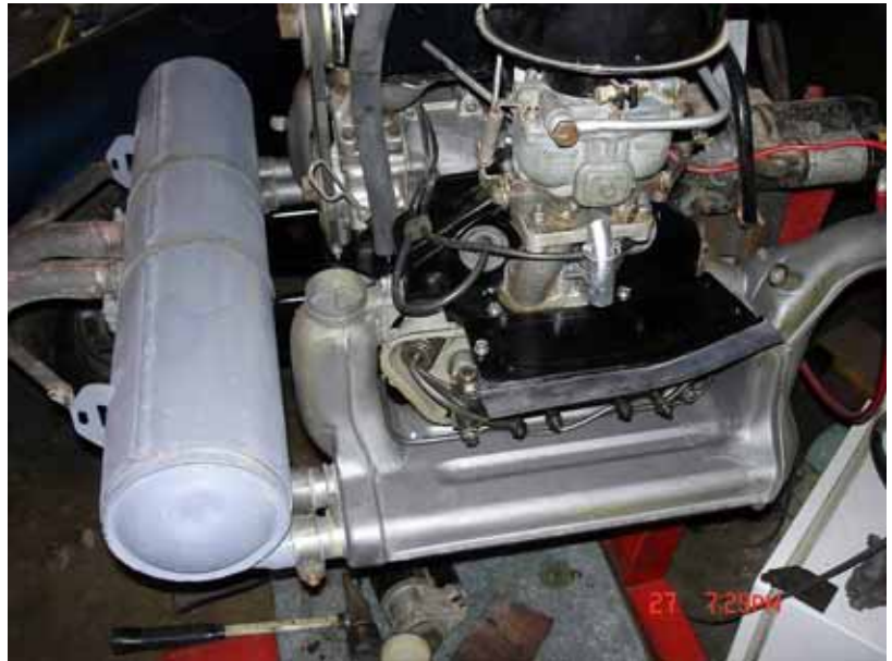
Right-side of motor shows NOS Euro heat exchanger and carburetor pre-heat tube looking showroom new.
